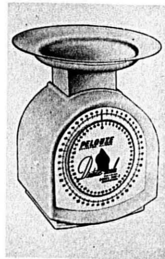
Automatically weighs each food portion and computes total weight of meal. Two simple dials do the trick. Inner dial shows weight of each individual portion, outer dial automatically totalizes entire meal. One-piece white plastic housing makes cleaning easy. Scale is sensitive to 1/2 gram. Light-weight plate provided makes full capacity of 500 grams available. Overloads will not damage the Pelouze Scale. For complete information, write the manufacturer.
